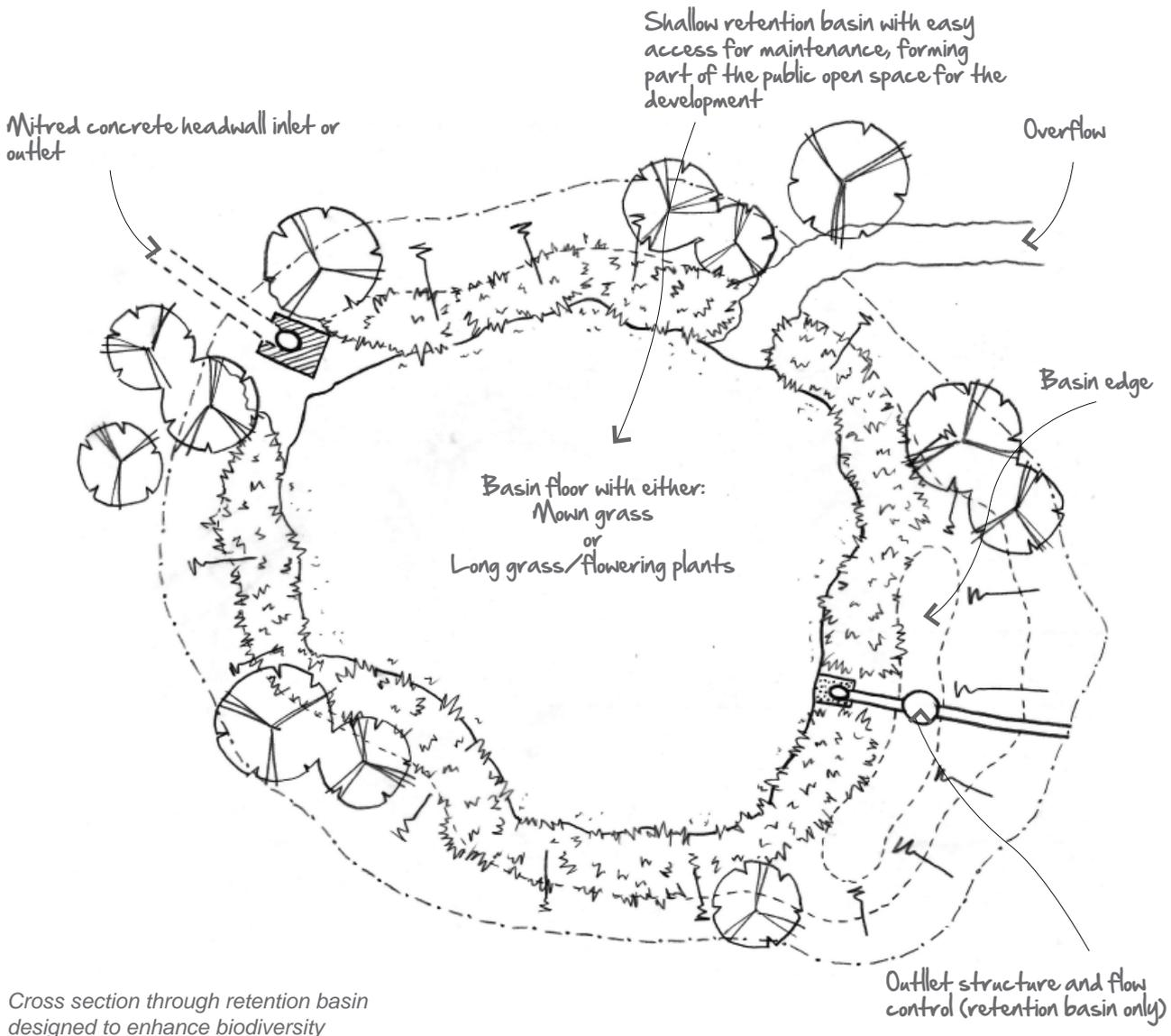
Cross section through retention basin designed to enhance biodiversity
