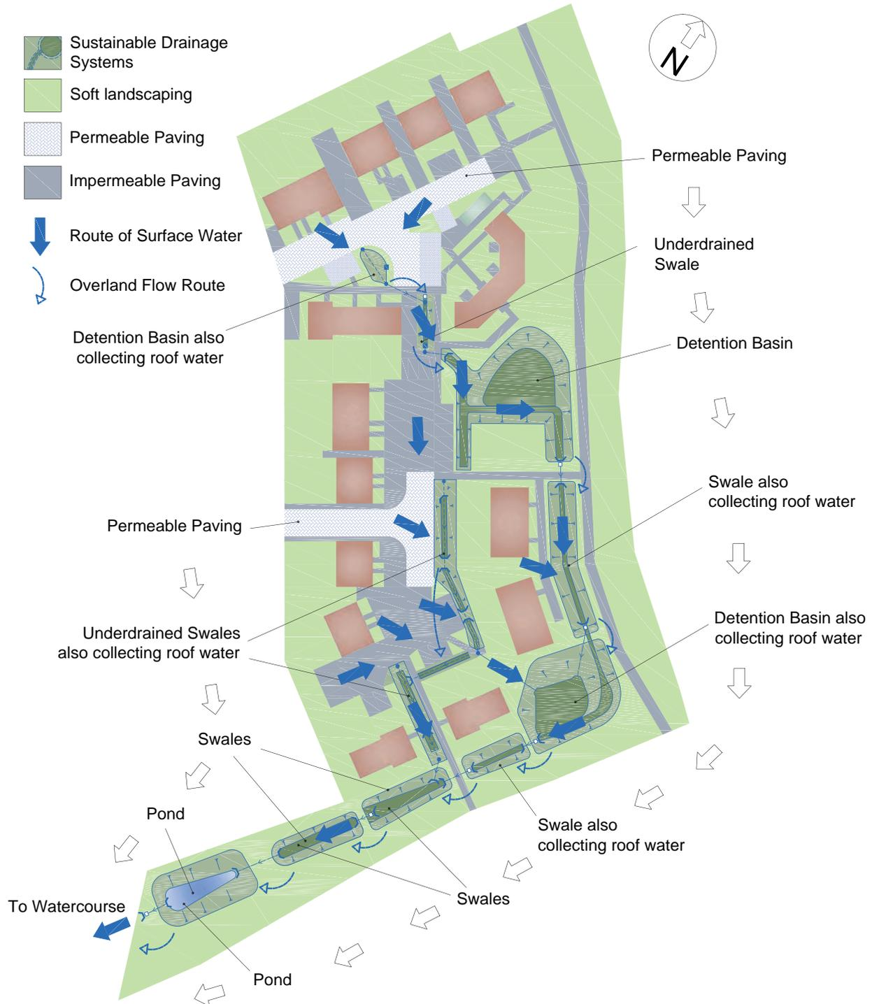
A habitat survey has shown that the SUDS provide a greater diversity than normal open space. The maintenance of the SUDS has been incorporated into the day to day maintenance of the open space. The extra costs for maintaining the SUDS are minimal when compared to those for maintaining normal open spaces.
