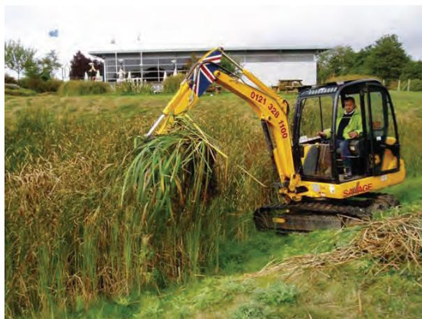
*Managing wetland vegetation with a mini excavator. Larger excavators should not be necessary, motorway service area, M42*
